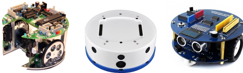
Figure 3.2: Example of mobile robot platforms under analysis: ct-Bot (left), Khepera IV (middle) and AlphasBot2 (right).
