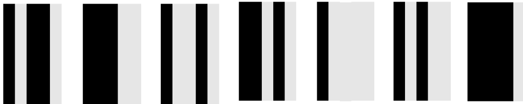
Figure 4.2: Barcodes placed on the ground environment (the barcodes associated with checkpoints 1 to 6 are represented from left to right; the GOAL checkpoint is the rightmost).
