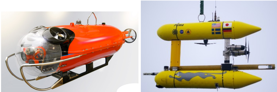
Figure 2.4: Pluto Plus - countermining (left) and WHOI SeaBED - collect sonar and optical images of the seafloor (right).
